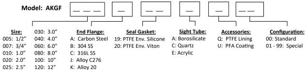
\*Contact ARCHON for additional material options, temperature ratings or special configurations.
