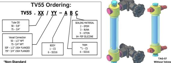
The TAG-57 model level gauge along with TV-55 valves is a sturdy alternative to the tubular gauge with guard rods. This gauge has a polycarbonate tube to protect the glass from breakage at the same time providing full view of the process fluid inside the glass tube. It provides more visible length for the same vessel C-C than direct mounting of the glass to the valves.
