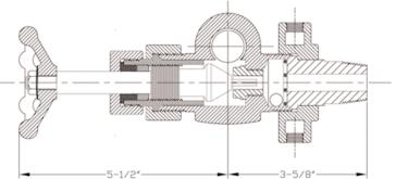
ARCHON Heated Gauges and Gauge Cocks are designed to meet certain conditions where heating is necessary to keep liquids flowing more freely to provide an accurate reading of the liquid level.
